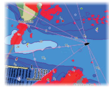
Radar overlay on a chart
